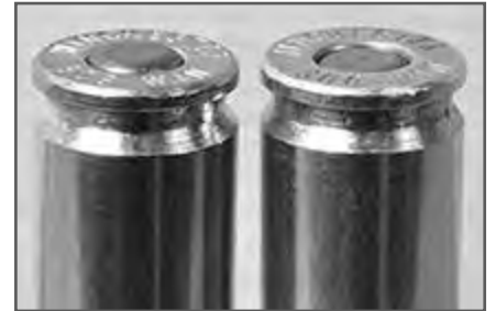
Example 12: Primer on left is not seated deeply enough
