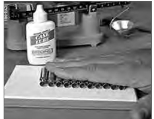
Example 4: Applying Case Lube
