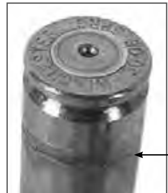
Example 2: Case Head Separation
