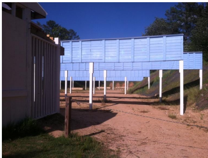
Pistol Range Baffles – A View Downrange:
