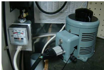
Variac to adjust 115VAC input voltage which adjusts output HV levels
