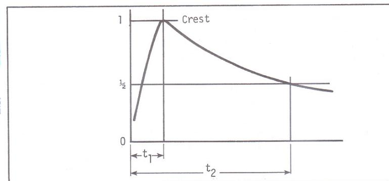
Definition of a Stroke Waveshape in Terms of its Time to Crest and its Time to Return to Half Crest ( $t_1 \times t_2$ ).
