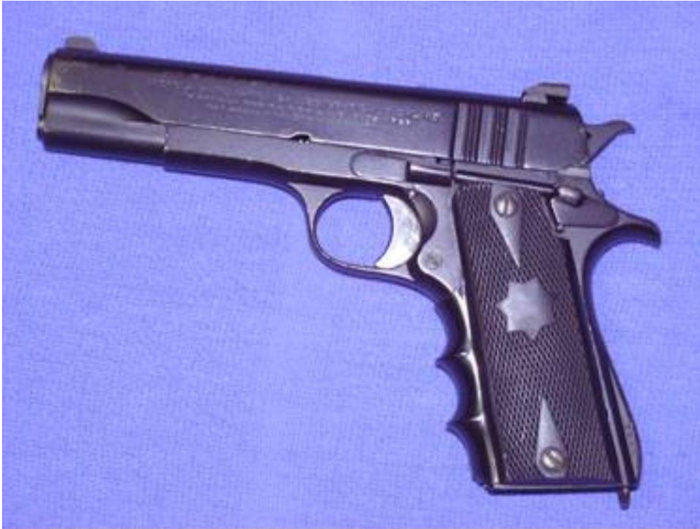
Figure 1: A formerly inoperable Ballester-Rigaud that was returned to serviceable condition by adding MMC sights (the rear sight is secured with .005" shim stock) and a shiny donor trigger/sear bar from a Star PD to replace the broken original. Although not visible, a M1911 barrel bushing, recoil plug, and recoil spring were also used to replace the missing originals. Note the late-style Argentine rubber grips that greatly resemble the old Bianchi Lightning grips once offered for the M1911 pistols. The finish is someone's poor attempt to duplicate a Suncorite or "stoving" finish as seen on many British military firearms. This old warhorse was purchased and repaired for less than $200, making it an ideal truck gun.
